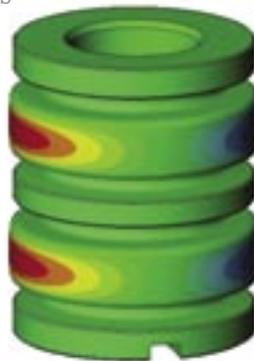
solid model without any translation or hand-off step required. This overcomes the old process of exporting the design file in a neutral format, like IGES or STEP, then accessing that neutral file with a free-standing FEA program.
