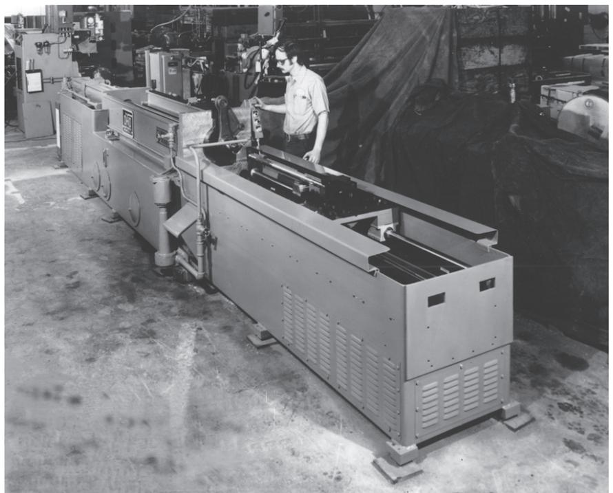
of the internal broaches. It produces close-tolerance parts and smooth surface finishes in high production applications.
