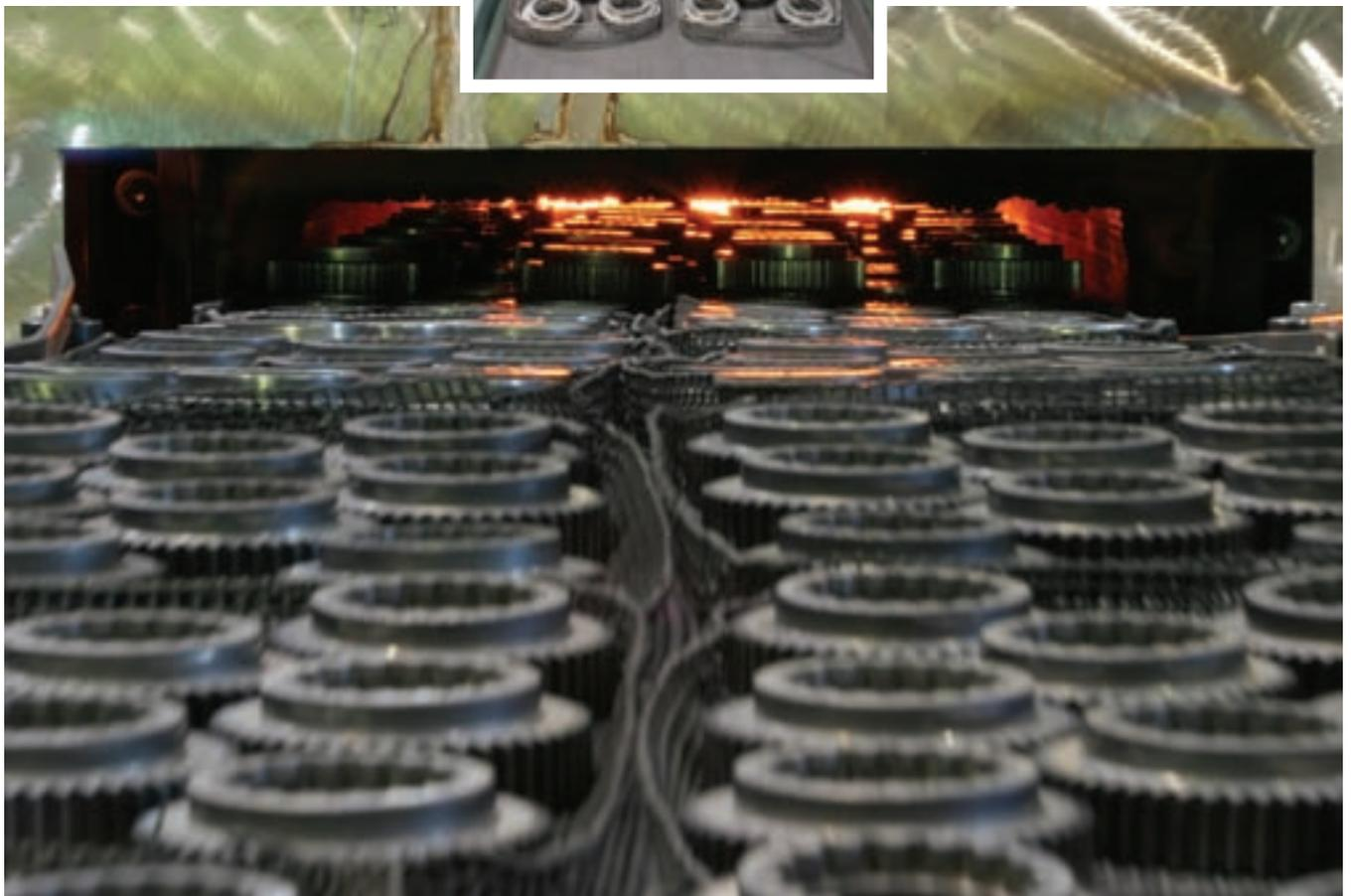
Newly formed gears are sintered on 65' continuous belt furnaces at a temperature over 2,000° F.
