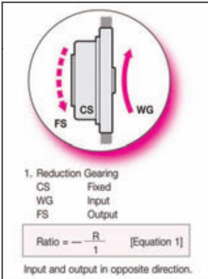
continuously moving elliptical form or wave-like motion to the flexspline. This causes the meshing of the external teeth of the flexspline with the internal teeth of the circular spline at their two equidistant points of engagement. This meshing progresses in a continuous rolling fashion. It also allows for a full tooth disengagement at the two points along the minor axis of the wave generator.
