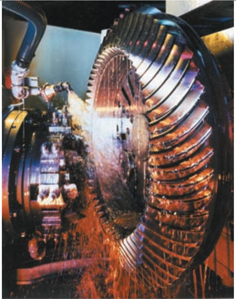
Overton's recent purchase of Illinois Gear gives the company the ability to manufacture large-diameter spiral bevel gears.
