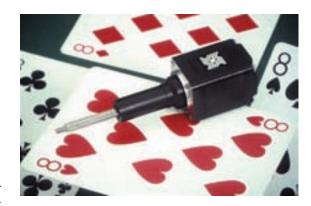
Built for several million cycles and superior performance, the Size 8 linear actuator features engineering thermoplastics in the rotor drive nut and a stainless steel acme lead screw. With this patented design, quietness and maintenance are ensured, according to HSI's press release. This captive hybrid linear actuator is available with resolutions ranging from 0.0015-0.04 mm and delivers thrusts up to 4.5 kg.
