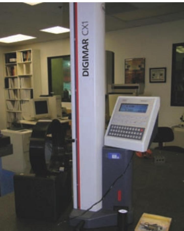
Gerhardt Gear says its CX1's accuracy is  $\pm 0.0001$ ". Specialties of the CX1 include the measuring of planes, grooves, bores and shafts as well as the calculations of distances and symmetries. Max.-min. measurements are supported, as are perpendicularity measurements in conjunction with a digital dial indicator. Canned routines for basic features and simplified teach-and-learn techniques make it easier to program for a variety of measurement tasks.
