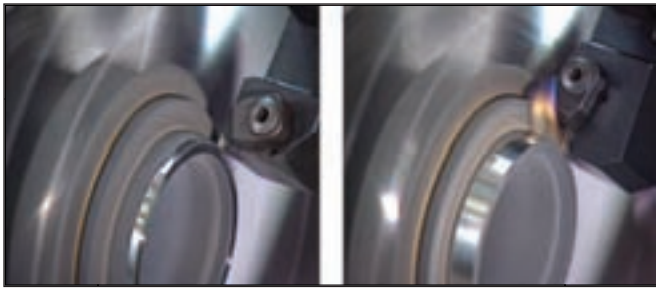
Figure 7—Manufacturers have several options for machining the synchromesh taper.
