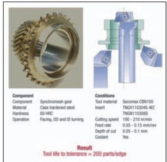
Figure 14—The preferred option at one manufacturer is to use plunging for the tapered cone and front face and wiper inserts for the bore and rear face.
