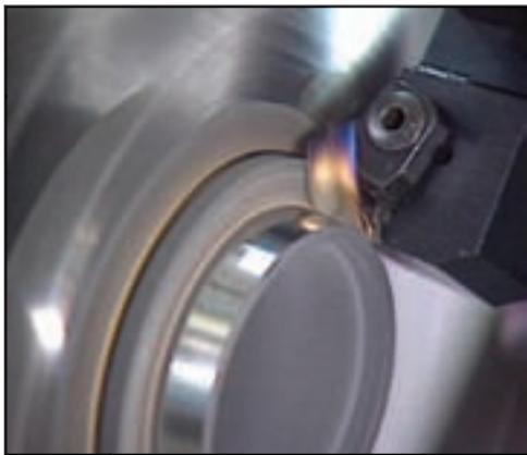
Figure 8—Parameters for plunge turning a synchromesh taper.
