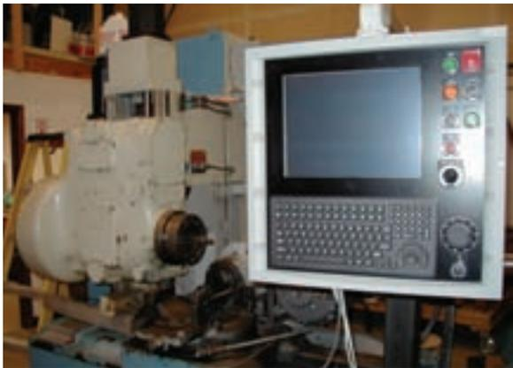
NOVA Systems has introduced a program for retrofitting gear cutting machines and aging CNC controls with state-of-the-art digital motion control.
