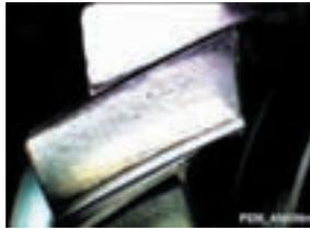
**Figure 8**—MEGAGEAR, 19 teeth, 4 NDP, 35° PA, 30° helix angle; showed some wear after 50 million load cycles at 1,686 hp.
