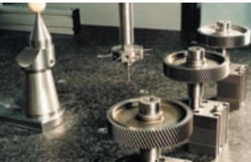
Nelson added that the company had initially looked at a dedicated gear checking machine. "For the money, the CMM was a better investment for us," he says. "The PMM-C can check gears with an extremely high degree of accuracy, plus it has the size and measuring range that allows us to inspect our prismatic parts as well."
