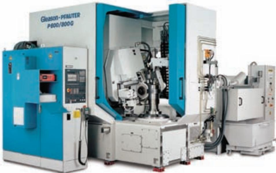
The latest modules feature one for adaptive process control. Available since the second half of 2005, the software reduces grinding time by running the grinding wheel at its normal operating feed rate only during actual contact between wheel and workpiece.
