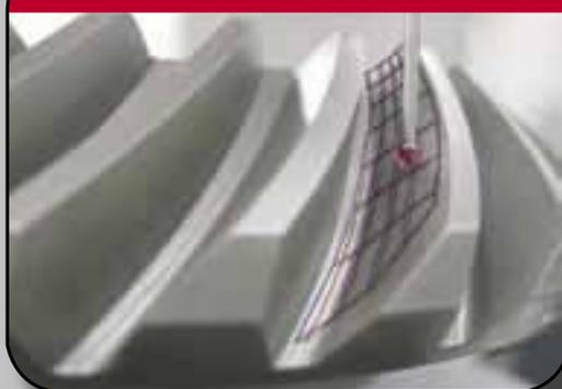
Topological Inspection for spiral angles and pressure angles:
