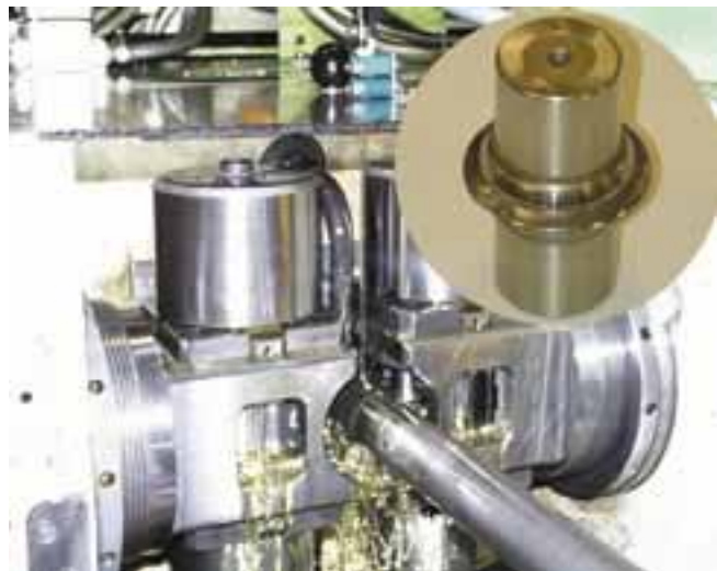
Tool monitoring systems from Nordmann can help detect problems before they occur, preventing expensive tool breakage like the chipped rolling die shown in the inset above.
