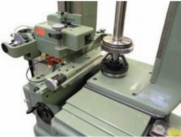
Figure 8—Maag PH 60 involute and lead tester, around 1962.
