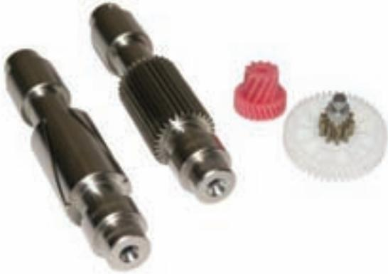
Figure 19—IC artifacts (m=0.8) for small gears.
