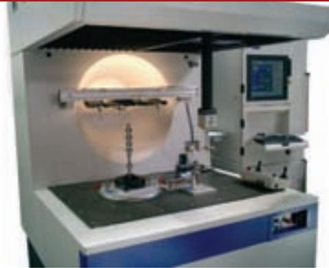
Figure 17— Zeiss Gagemax universal 3-D coordinate measuring machine with rotary table for gear measuring.
