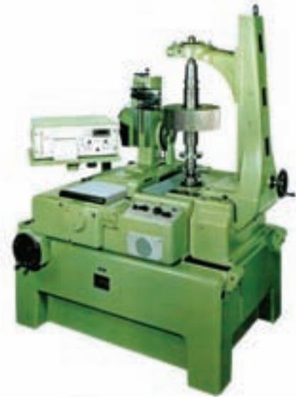
Figure 9—Maag SP 60 variable involute and lead gear tester, 1968.
