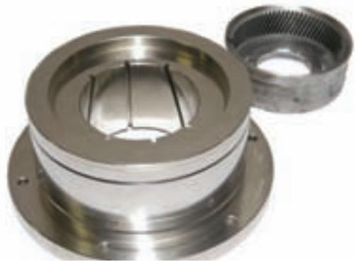
Figure 20—IC artifacts (m=2) for medium-sized gears.
