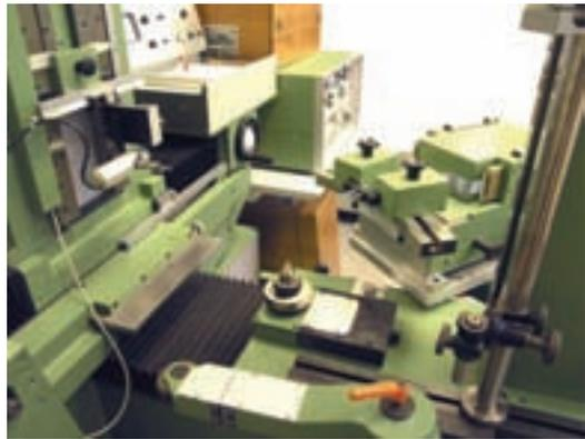
Figure 15— Höfler EFR S gear testing machine for involute, lead, pitch and runout, 1976.
