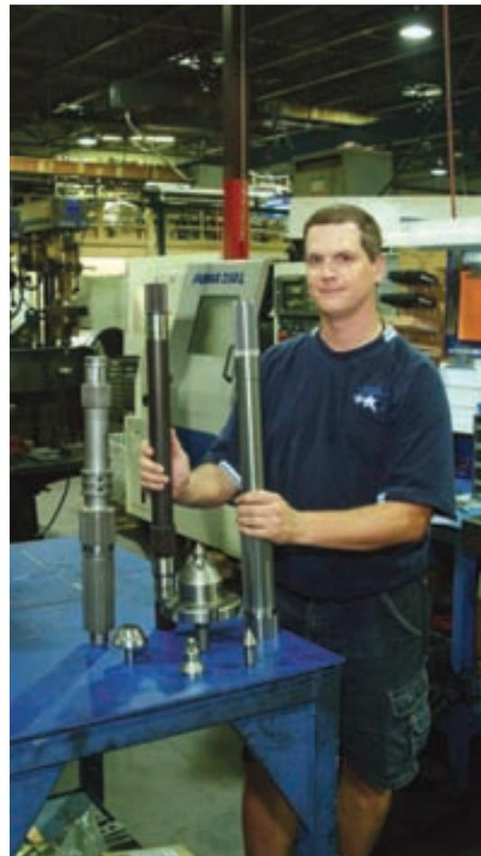
Keith Mallek, applications engineer with United Gear & Assembly, is holding two of the longer shafts the company manufactures. In addition to the shafts, the face driver and the live center pin used to turn these parts are shown in the foreground.
