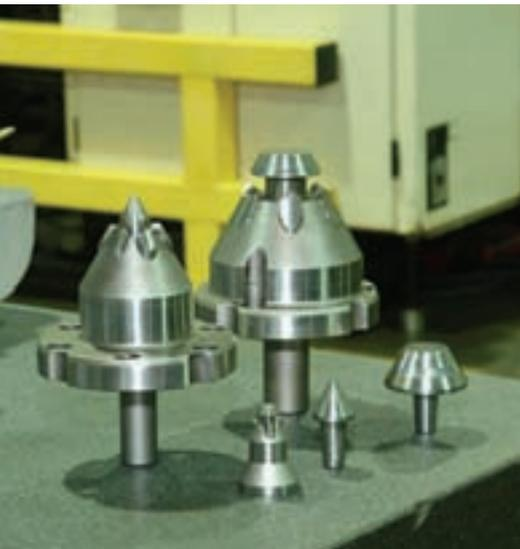
The face driver on the left is a Neidlein Model D-4. The other is a Model D-6. The tips on the right and in the middle are tips that United Gear can interchange on the RNW ultra live center. These are stock centers, but with these tips the company can run about 150 different part numbers just by changing the center pins. The third part in front is a replacement part for the face driver. Four extra ones were made so if one breaks they can be changed out in about five minutes.
