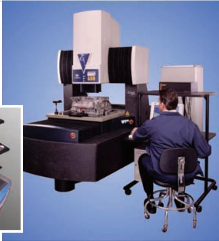
The SmartScope Quest 650 from Optical Gaging Products is a programmable five-axis measuring system for large volume dimensional metrology. A motorized, heavy-duty dual rotary indexer allows SmartScope Quest sensors to measure features anywhere on complex parts. OGP *MeasureMind* metrology software supports simultaneous five-axis motion, keeping the coordinate system aligned with the rotating part. The automatic system measures parts such as turbine blades, vanes and air folds.
