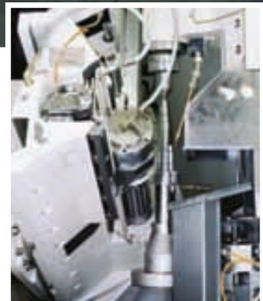
With the modules integrated, the CNC hobbers can chamfer and deburr spur and helical gears, creating a fully automated system for use in mass production.
