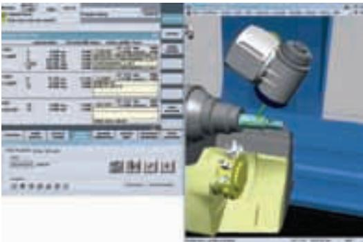
Index Corp. has upgraded its machine controls to include a virtual machine function, which fully simulates, on a PC, all machine motions and functions related to any machine program.
