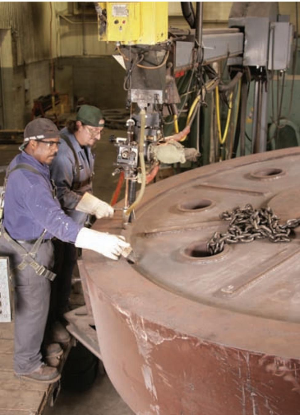
Horsburgh & Scott welders Barry McDowell (front) and Dave Evans (back) create fabricated gears from three components—the outer ring, from which the gear teeth are cut; the inner hub; and the internal webbing that acts as the spokes of the wheel.
